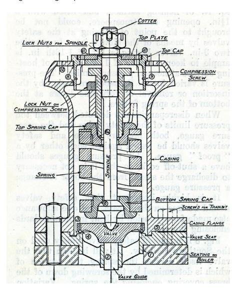
If a safety valve is suspected to be defective or the boiler pressure rises above the red line marked on the locomotives pressure gauge it should be reported to the Locomotive Department Person In Charge. Only competent staff must carry out work on safety valves.
