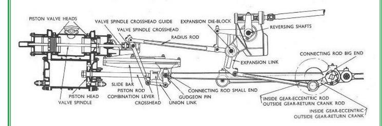
Normally the bottom of the link is used for fore gear and the top of the link for back gear working, giving a direct movement for fore gear and indirect movement for back gear.
