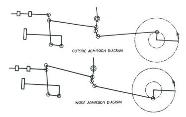
Variations of this gear are used to operate outside cylinders with the valve gear inside as on former G.W.R locomotives, also outside valve to operate inside cylinders as on the later builds of former L.M.SR. 4-6-2. Another variation is that used on former L.N.E.R 3-cylinder locomotives in which the Walschaerts' valve gear for the outside cylinders operate the inside cylinder through a system of levers.
